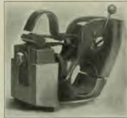
FIG. 4. BRUSH AND HOLDER OF WESTINGHOUSE MOTOR
